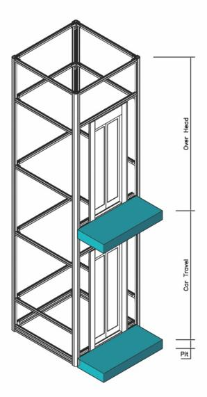
Shaft and shaft structure dimensions depend on access number and layout.
